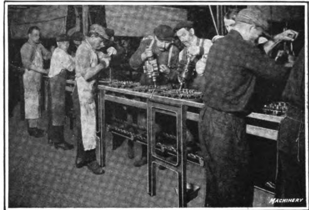
Fig. 27—In this case, the magnetic generator unit of the motor is carried on an endless belt conveyor, and men with power-driven wrenches are screwing up the nuts. Attention is called to the large number of men at work; this is typical of the intensive production methods in the Ford Motor Co.'s shops
